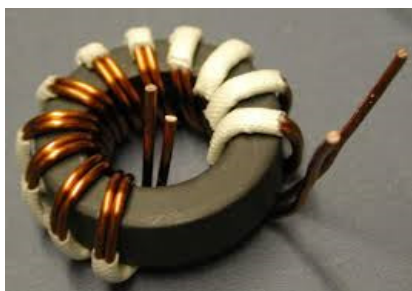
Bifilar Winding Technique Figure 8
