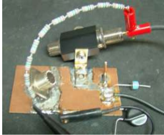
Figure 18 - Gas Tube Test Fixture
